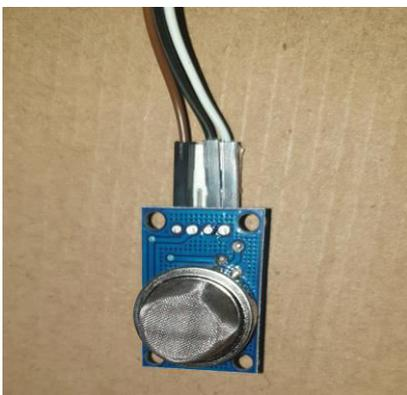
It can sense the dry gases present in the toilets such as  $\text{NH}_3$ ,  $\text{CO}_2$ ,  $\text{CH}_4$ ,  $\text{H}_2\text{S}$ , etc. By taking those gases leads to Nausea, Drowsiness, instant loss of awareness, etc. After sensing the unwanted gases, it can blink the red light. Then the sweeper can clean it by using particular Cleaning Agents.
